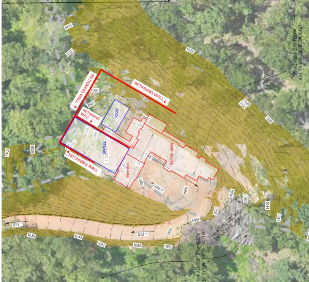
Figure 2: Proposed Improvements and Critical Slopes
